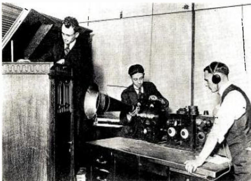
This DeForest Model OT-10 transmitter, shown here as it picked up phonograph music, worked on Aug. 20, 1920, the day broadcasting was born at WWJ
